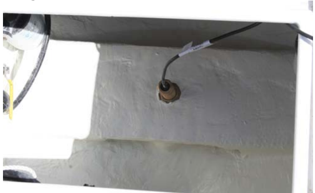
Extra Reinforcement in the Bilge, then Gel Coated
