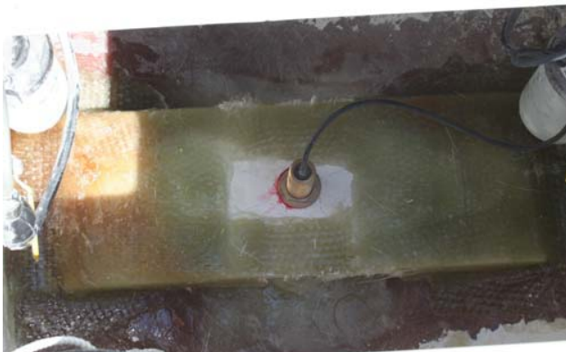
Extra Reinforcement in the Bilge, then Gel Coated
