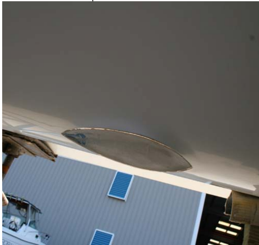
New Transducer Epoxied in and Gel Coated - SWEET!!!
