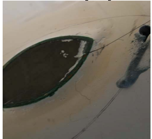
The old transducer getting cut out
